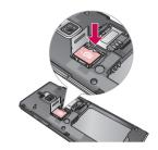
The slot has to be opened by pulling the metal cover upwards.
