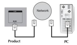
Connect the LAN cable and install the eZ-Net Manager program on the CD-ROM.
