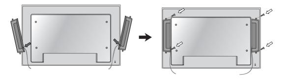
After installing your speakers, use holders and cable ties to organize the speaker cables.
