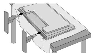
**3.** Use the screws to secure the stand on the rear side of the product as shown in the diagram.
