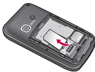
To remove the USIM card
