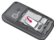
To insert the USIM card
