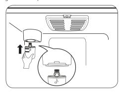
3. Push the water filter up into the filter receptacle and rotate it clockwise to lock it into place. Once installed correctly, the lock symbol \( \text{\text{c}}\) should be facing you and you should not be able to rotate the filter clockwise any more.
