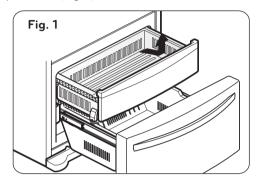
To reinstall, pull out and fully extend both rails. Insert the end of rib in the bracket at left and right. Making sure that the guides at the front are lined up properly, gently push downon both sides (Fig. 2)
