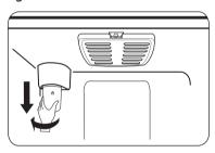
For filter replacement, remove old filter by turning it counterclockwise and pulling it down.
