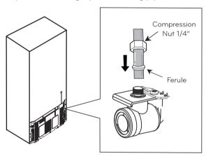
Hold on to the pipe from the handles or grabbers located behind the refrigerator, loosing first the bolt holding the handle. Afterwards, insert pipe into the hole and tighten bolt to finalize.
