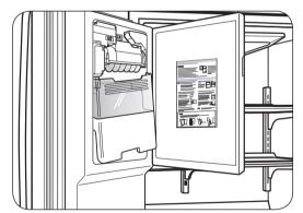
To remove the in-door ice bin, grip the front handle, slightly lift the lower part, and slowly pull out the bin as shown.
