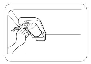
Press the push button to open the filter cover.
