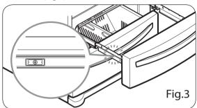
• With the drawer pulled out to full extension, insert the drawer and ice bin in the rail. (Fig. 4)
