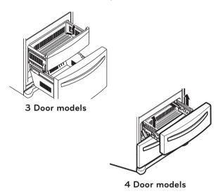
To reinstall, pull out and fully extend both rails. Insert the end of rib in the bracket at left and right. Making sure that the guides at the front are lined up properly, gently push down on both sides.
