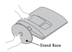
Turn the **Stand Base Lock** through 90° to separate the stand base from the stand body.
