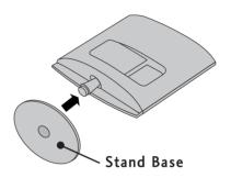
Turn the **Stand Base Lock** through 90° to fix the stand base to the stand body.
