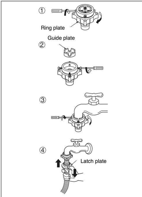
1. Unscrew the adapter ring plate and the 4 adapter retaining screws.
