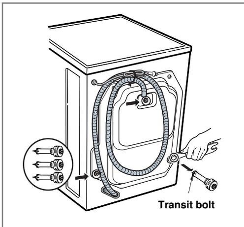
1. Unscrew the 3 bolts with the spanner supplied.
