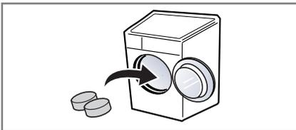
1. Open the door and put tablets into the drum.
