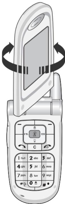
You can rotate LCD clockwise an angle of 90 degrees and counter-clockwise an angle of 180 degrees. However, if you turn it by force, it can cause serious damage.
