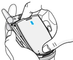
1. Position the lugs on the bottom of the battery into the retaining holder.
