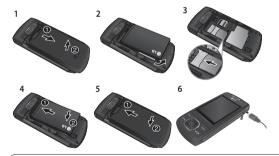
MARNING: Do not remove the battery when the phone is switched on, as this may damage the phone.
