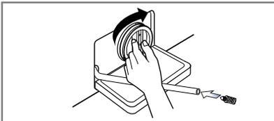
4. After cleaning, turn the pump filter and insert
