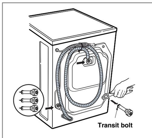
1. Unscrew the 3 bolts with the spanner supplied.
