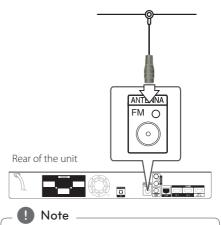
After connecting the FM wire antenna, keep it as horizontal as possible. Be sure to fully extend the FM wire antenna.
