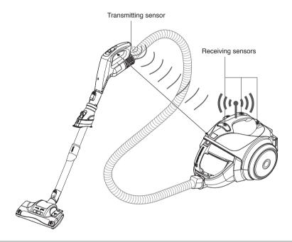
When using vacuum cleaner, be careful not to block the transmitting sensor by wall or body. If transmitting sensor was blocked, FOLLOW ME function cannot work properly.
