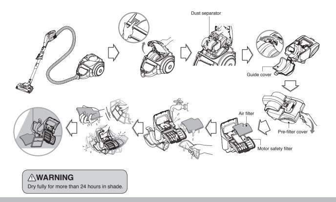
If suction power is decreased after cleaning dust tank, clean air filter and motor safety filter.
