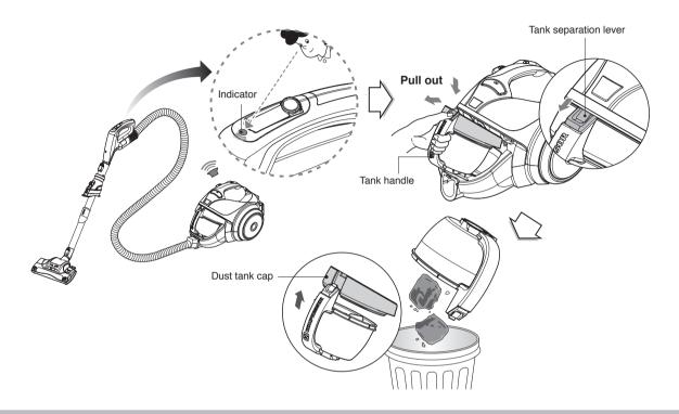
The dust tank needs emptying when indicator light is on.
