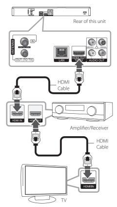
Connect the amplifier's HDMI output jack to HDMI input jack on your TV using a HDMI cable if your amplifier has HDMI output jack.
