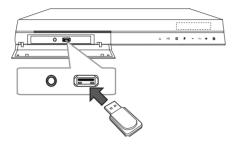
Removing the USB Device from the unit
