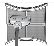
Clean the filter. (Replace the filter if it is damaged.)
