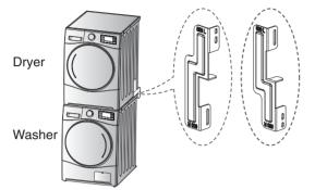
This dryer may only be stacked on top of an LG washer. DO NOT attempt to stack this dryer on any other washer, as damage, injury or property damage could result.
