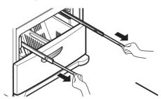
2 Grasp the drawer on each side and hook the door supports (1) into the rail tabs (2) located on both sides.
