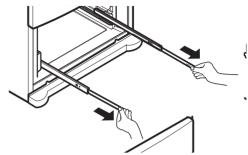
2 Grasp the drawer on each side and hook the door supports (1) into the rail tabs (2) located on both sides.
