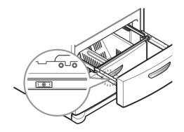
3 Grasp the drawer on each side and pull it up to separate it from the rails.
