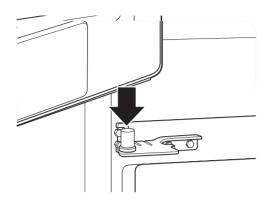
1 Lower the door onto the middle hinge pin.
