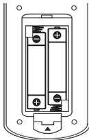
Remove the battery cover on the rear of the Remote Control, and insert one (size AAA) battery with  $\oplus$  and  $\ominus$  matched correctly.
