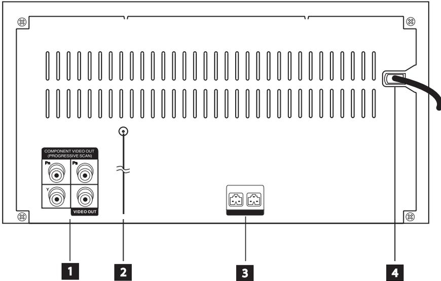
**1 COMPONENT VIDEO (Y PB PR) OUTPUT (PROGRESSIVE SCAN)**
