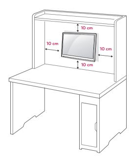
If you intend to mount the TV to a wall, attach Wall mounting interface (optional parts) to the back of
