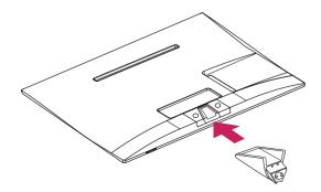
3 Attach the **Stand Base** from the **Stand Body** by turning the screw to the right with a **Coin**.
