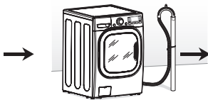
Connecting the drain line
