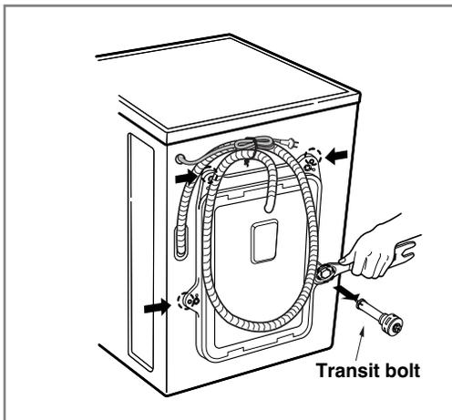
1. Unscrew the 4 bolts with the spanner supplied.
