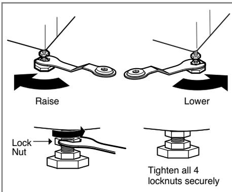
2. If the floor is uneven, turn the adjustable feet as required. (do not insert pieces of wood etc. under the feet)
