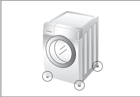
1. Leveling the washing machine properly prevents excessive noise and vibration. Install the appliance on a solid and level floor surface, preferably in a corner of the room.
