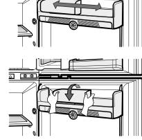
How to remove the cover for cleaning
