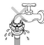
**Screw Type****1 Attach the water supply hose to the tap.**
