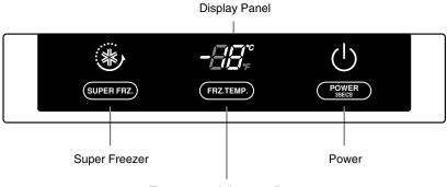
Temperature Adjustment Button for Freezer Compartment
