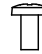
Bracket Screw 2EA, M4 x 8 (Only 32/42LA61**) 2EA, P4 x 8 (Only 50LA61**) (See p.16)
