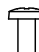
Bracket Screw 2EA, M4 x 8 (Only 32/42LA61**) 2EA, P4 x 8 (Only 50LA61**) (See p.16)
