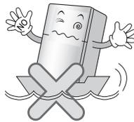
**Install the refrigerator on the solid and level floor.**
