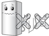
**Prevent the power cord from being squeezed or imprinted if the refrigerator is pushed in after the power plug is extracted during the installation.**
