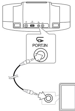
1. Raccordez l'appareil portable sur
