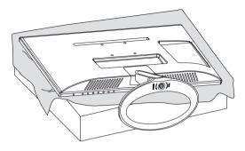
3 Turn the screw to the left, and then pull out the **Stand Base** from the **Stand Body**.
