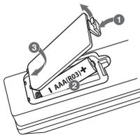
Detach the battery cover on the rear of the remote control and insert two R03 (size AAA) batteries with  $\oplus$  and  $\ominus$  aligned correctly.
