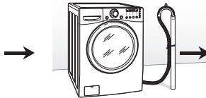
Connecting the drain line
