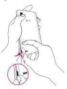
2 Slide the SIM card into the SIM card slot. Make sure the gold contact area on the card is facing downwards.
