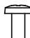
Bracket Screw 2EA, M4 x 8 (Only 32/42LA62**, 32/42LA64**, 32/42LA66**, 32LN56**, 32/42LN571*, 32/42LN61**) (See p. 19)
