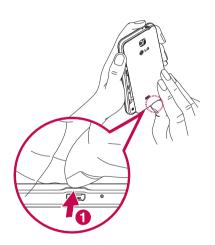
2 Slide the Micro-USIM card into slot as shown in the figure. Make sure the gold contact area on the Micro-USIM card is facing downwards.
