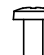
Bracket Screw 2EA, P4 x 8 (Only 47/50LA62**, 47/50LA64**, 47/50LA66**, 47LA71**, 47/50LN571*, 47LN61**) (See p. 19)
