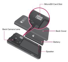
NOTICE The NFC antenna for this model is on the back cover. This back cover is the only one that is offered with the model.
