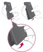
2. Insert the battery into place by aligning the gold contacts on the battery and the phone • and pressing it down until it clicks into place •.
