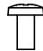
Bracket Screw 2EA, M4 x 8 (Only 32/39/42LA62**, 32/42LA64**, 32/42LA66**, 32/39LN56**, 32/42LN570T, 32/42LN571*, 32/42LN61**) (See p.20)
