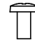
Bracket Screw 2EA, P4 x 8 (Only 47/50LA62**, 47/50LA64**, 47/50LA66**, 47LA71**, 47/50LN570T, 47/50LN571*, 47LN61**) (See p.20)
