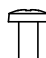
Bracket Screw 2EA, M4 x 8 (Only 32/42LA62**, 32/42LA64**, 32/42LA66**, 32/42LN571*) (See p. 19)
