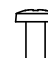
Bracket Screw 2EA, P4 x 8 (Only 47/50LA62**, 47/50LA64**, 47/50LA66**, 47/50LN571*) (See p. 19)
