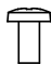
Bracket Screw 2EA, M4 x 8 (Only 32/39/42LA62**, 32/42LA64**, 32/42LA66**, 32/39LN56**, 32/42LN570T, 32/42LN571*, 32/42LN61**) (See p.20)
