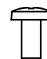
Bracket Screw 2EA, P4 x 8 (Only 47/50LA62**, 47/50LA64**, 47/50LA66**, 47LA71**, 47/50LN570T, 47/50LN571*, 47LN61**) (See p.20)
