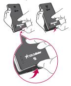
Slide the SIM card into the SIM card slot. Make sure the gold contact area on the card is facing downwards.
