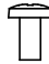
Bracket Screw 2EA, M4 x 8 (Only 32/42LA62**, 32/42LA64**, 32/42LA66**, 32/42LN571*) (See p. 18)
