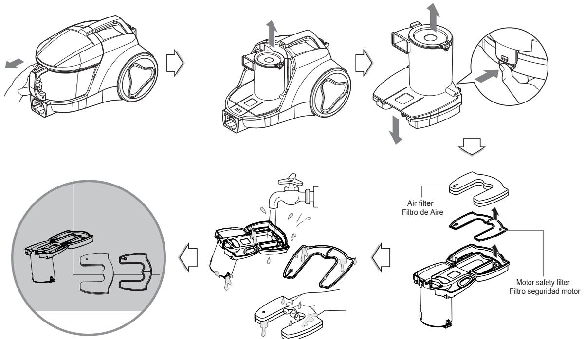
If suction power is decreased after cleaning dust tank, clean air filter and motor safety filter.
