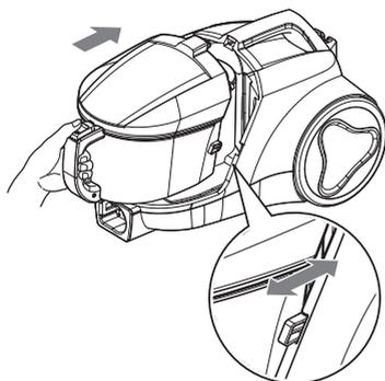
Slide the tank on product to match the tank ribs to groove of body.
