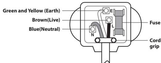
As the colours of the wires in the mains lead of this apparatus may not correspond with the coloured markings identifying the terminals in your plug, proceed as follows:
