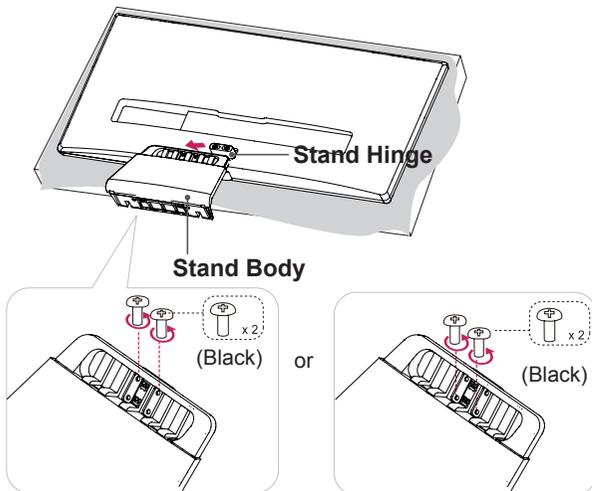
4 Remove the two screws from the Stand Base. Remove the Stand Base from the Stand Body.
