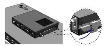
In order to watch video on a monitor, you need to use a D-sub cable or an HDMI cable to connect the NC1000 to a monitor.
