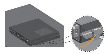
To view images on the monitor, you need to connect NC1100/NA1000/NA1100 to the monitor via a D-SUB, HDMI or DP cable.
