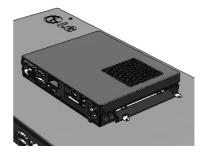
6 Use screws to secure the player and the Box Guide as shown below.
