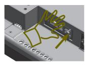
If card does not become fully inserted into the insertion direction. Hit by hand carefully to make fully connected.
