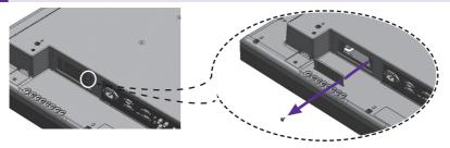
2 Attach the Box Guide to the rail slots, and press it upward.
