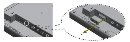
Attach the Box Guide to the rail slots, and press it upward.
