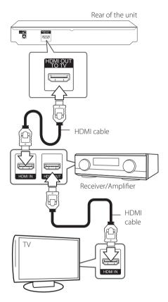
Connect the amplifier's HDMI output jack to HDMI input jack on your TV using an HDMI cable if your amplifier has HDMI output jack.
