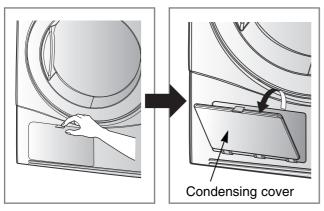
2. Open sealing cover by turning a locking lever.
