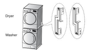
This dryer may only be stacked on top of an LG washer. DO NOT attempt to stack this dryer on any other washer, as damage, injury or property damage could result.
