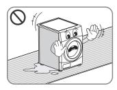
• If the dryer is installed on the carpet, it might be caused some damages by the ventilated air.
