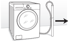
Connecting the drain line
