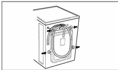
1. To prevent internal damage during transport, the special 4 bolts are locked. Before operating the washer, remove the bolts along with the rubber bungs.
