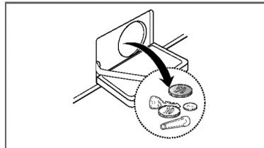
3. Remove any extraneous matter from the pump filter.
