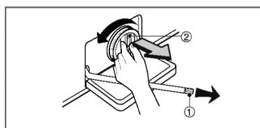
2. Unplug the drain plug (①), allowing the water to flow out. At this time use a vessel to prevent water flowing on to the floor. When water does not flow any more, turn the pump filter (②) open to the left.
