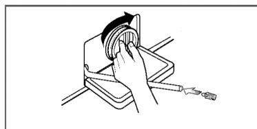
4. After cleaning turn the pump filter right till the end to meet white lines on the filter and pump body. Then insert the drain plug to the hose.
