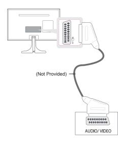
Transmits the video and audio signals from an external device to the TV set. Connect the external device and the TV set with the euro scart cable as shown.
