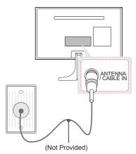
Connect the TV to a wall antenna socket with an RF cable (75  $\Omega). \label{eq:solution}$
