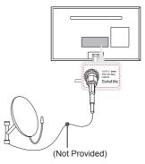
Connect the TV to a satellite dish to a satellite socket with a satellite RF cable (75  $\Omega$ ).
