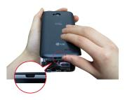
2. Insert the battery into the opening on the back on the phone, making sure the connectors align 1 and press down until it clicks into place 2.
